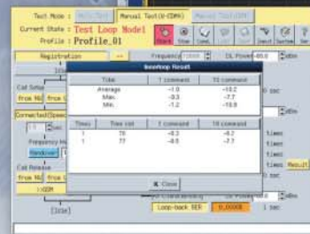
Inner loop power control
