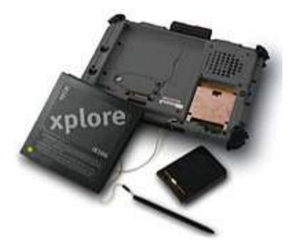
• Industry's highest capacity extended-life 68.5 Whr Li-Ion 10-cell battery provides up to 6.5 hours of operating time (Passmark Battery Test)
