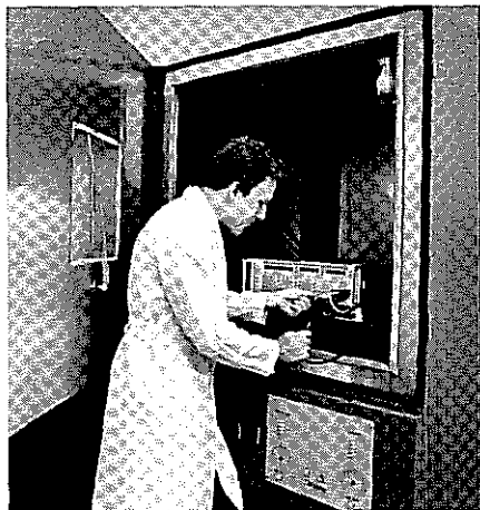
Figure 15. Every instrument is subjected to 72 hours of 50°C temperature cycling before shipment.
