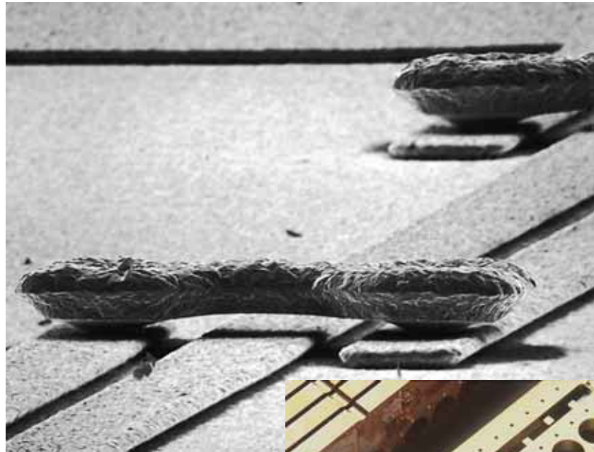
Airbridges is an ideal technique for implementing PCB crossovers with excellent high-frequency characteristics. The photo above has been taken with a scanning electron microscope and shows such an airbridge which is only 0.05 mm long.
