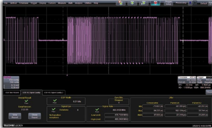
High-speed upstream signal quality test result.
