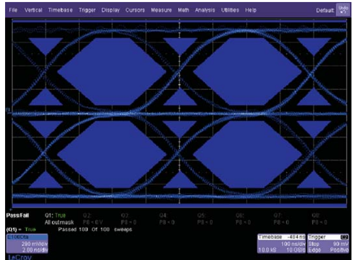
Figure 3: 100Base-TX twisted pair active output interface mask test result.
