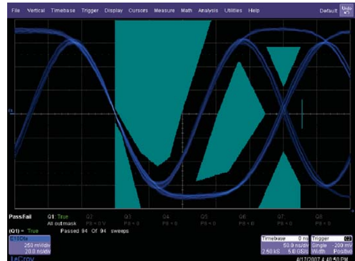
Figure 4: 10Base-T DOV External Mask Test
