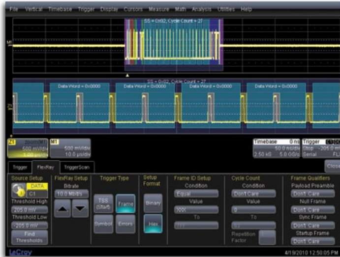
Trigger on every aspect of the FlexRay Frame as well as Symbols and Errors including FSS, BSS, FES, CRC, CID, CAS/MTS and Wakeup by selecting the appropriate boxes.
