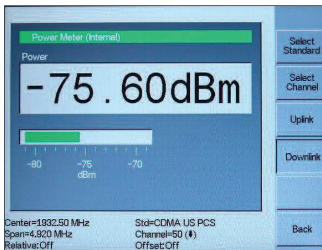
Figure 13. Power Meter Display (Site Master Platform)
