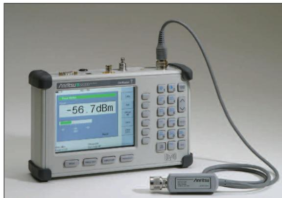
Figure 9. Option 5 Power Measurement
