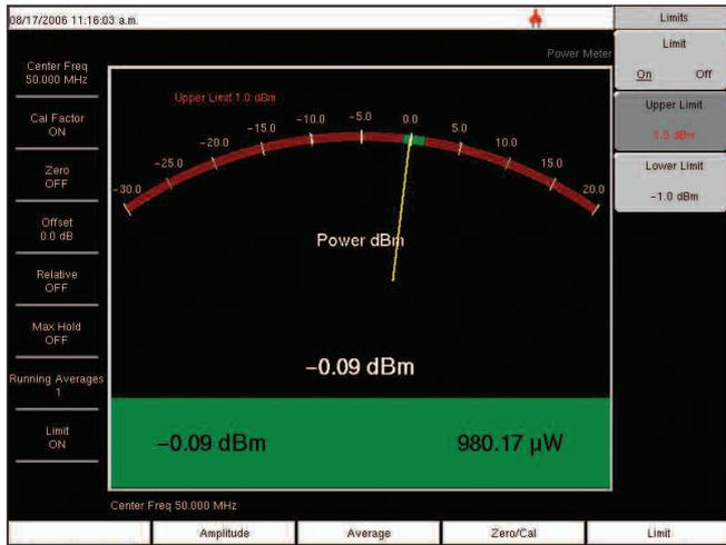
Figure 6. High Accuracy Power Meter display (MT8222A, MS272XB)
