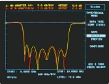
The Return Loss measurements (above) were created by the same bandpass filter. Measurement was performed with and without a test port adapter. Differences in the ripple display are caused by the vector error signal of the adapter's SWR reflection, which alternately adds and subtracts from the true return loss magnitude.
