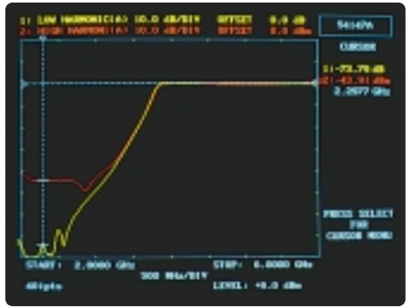
Errors due to source harmonics are most evident when testing wide band filters. As the source's fundamental frequency passes 2 GHz, the -33 dBc second harmonic is at 4 GHz – within the pass band of the wideband filter.
