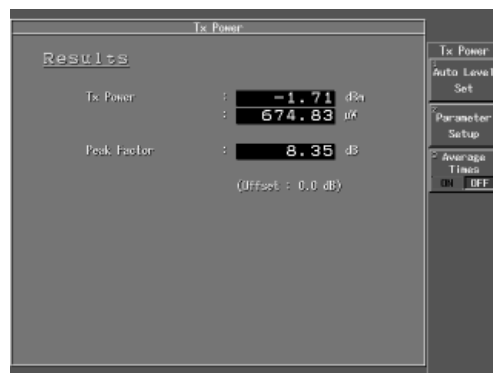
Sample of Tx Power measurement
